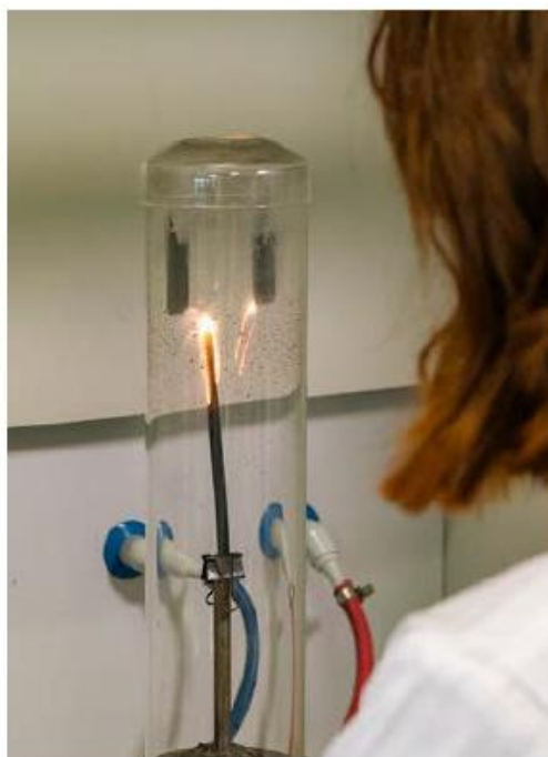
Oxygen index test, to assess the flammability of a material based on the percentage of oxygen present.
